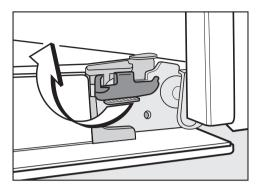
■ Flip both locking clamps back up as far as they will go into a horizontal position. Turn them as far as they will go into a horizontal position.
